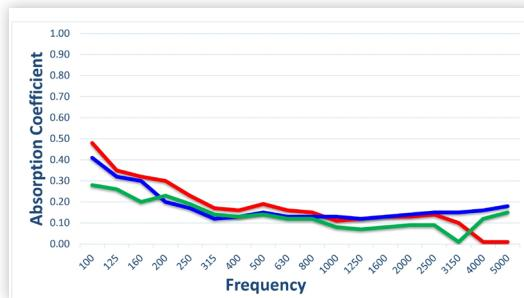
Blue = 4'x4' E-Mount Absorption Coefficient - NRC=0.15, SAA=0.15
