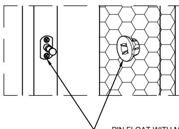
PIN FLOAT WITH MOUNTING PLATE AT MODEX CORNER TO BE MOUNTING WITH THE CONNECTOR AT FACE FRAME
